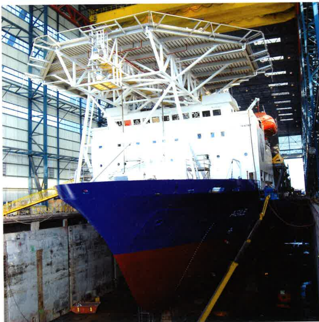
Scheldepoot's 215 metres long covered drydock made the conversion planning independent of weather
